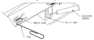
To avoid having ESD (electrostatic discharge) interfering with the operation of the reader, the reader casing shall be grounded. This can be accomplished be tying the mounting bracket to earth ground locally (e.g. grounded conduit). The reader has a four dip switch block which must be configured. All four switches must be in the OFF position. When looking into the back of the reader, all switches should be pushed away.
