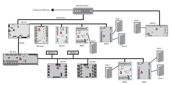
Note: The above specifications are based on the typical 12 volt reader drawing 125 mA. Reader power requirements vary between different models. Excessive voltage drop on long cable runs may require a larger cable gauge or powering the reader from a local power source. Refer to the power specification for the reader being installed.
