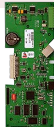
Mercury M5 Bridge designed for a direct retrofit /replacement of the CASI Micro5
